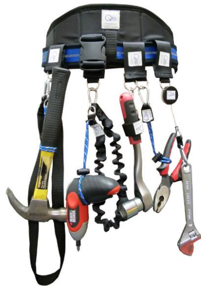
Figure 78 – Tool belt with lanyards on tools
