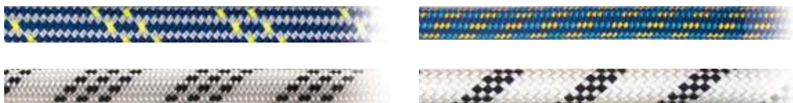
Figure 45 – Kernmantle static line examples
