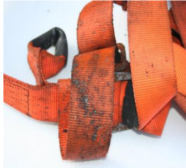
Figure 43 – Damage from contaminates
