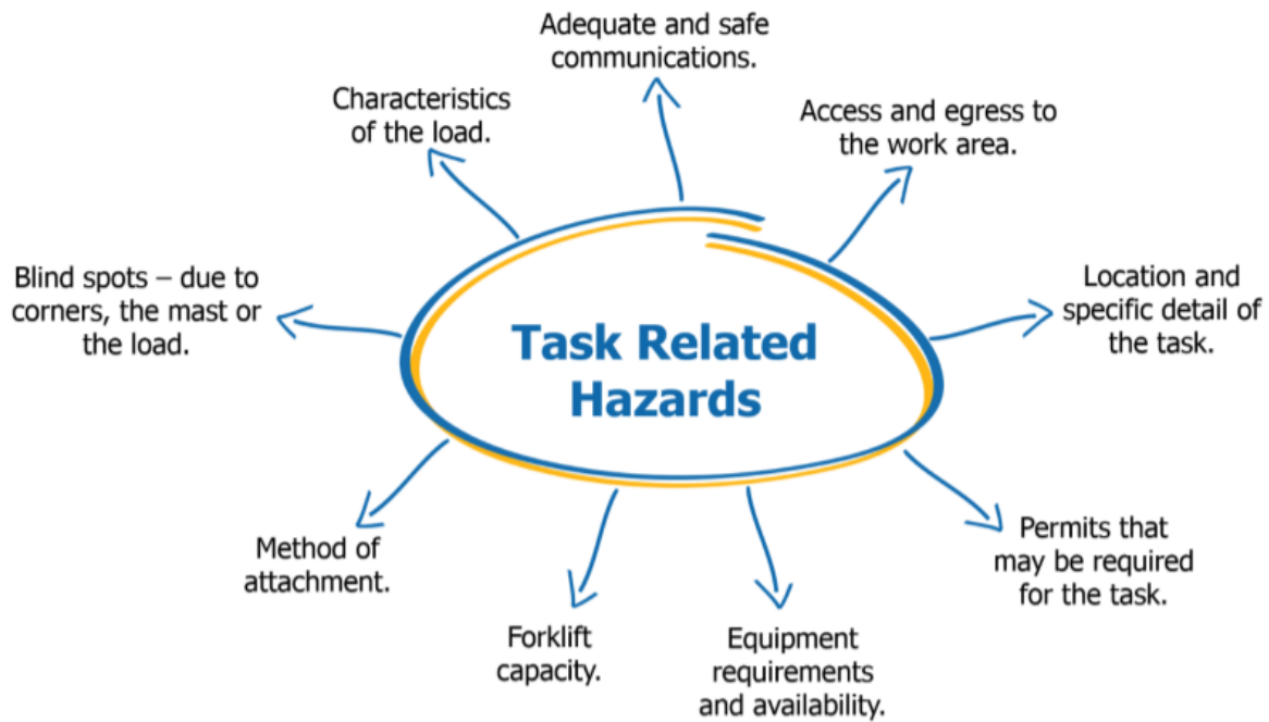
Figure 4 – Task Related Hazards
