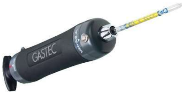
Figure 18 – Gas Sampling Pump with Glass Tube fitted
