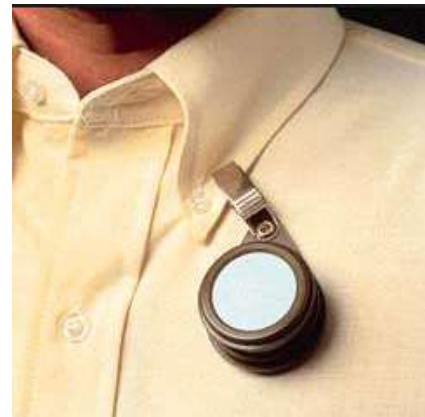
Figure 17 – Organic Vapour Air Monitor
