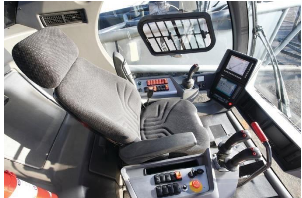
Figure 17 – Crane cabin and controls Check the Crane Logbook
