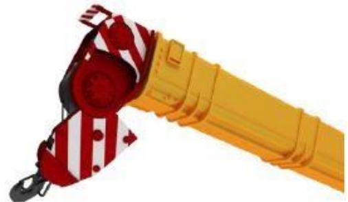
Figure 27 – Hook & Head Block
