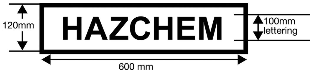
**Figure 13.1 Form and dimensions of outer warning placard**
